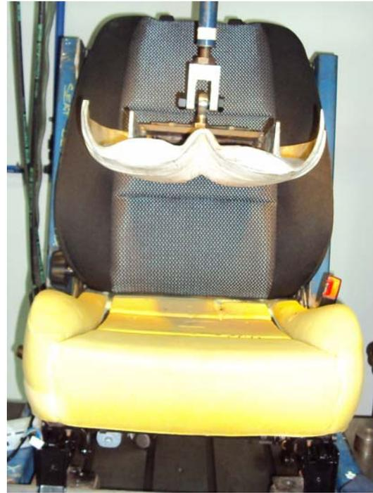
Figure 1: Seat indentation test on an untrimmed seat cushion, following FORD CETP 01.10-L-401.
