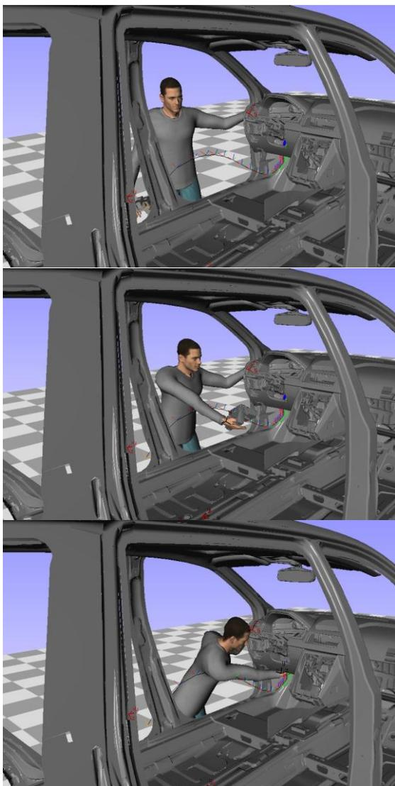
Figure 3. Snapshots from three states of installing the CEM box into its place.
