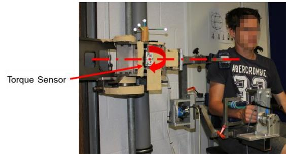
Figure 1: Shoulder joint torque measurement device
